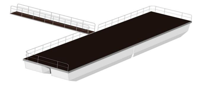
Landing pontoon for metropolitan line PROPELER in Bratislava with floats from a special plastic material L= 36 m, B= 8 m with superstructure designed for passenger services.
