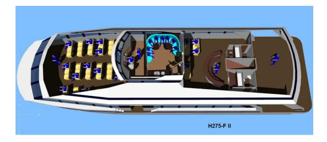
Base landing pontoon with floats from a special plastic material L=24 m, B=6 m with superstructure for passenger services designed for regional liner- and tourist transport.
