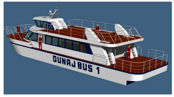
Exclusive fast catamaran JB275 RIVERCAT L=28 m, B=8 m, T= 0,8 m, propulsion machinery Arneson Surface Driver 2 x 450 kW, speed up to 65 km/h for 107 passengers + bicycles for tourist transport.
