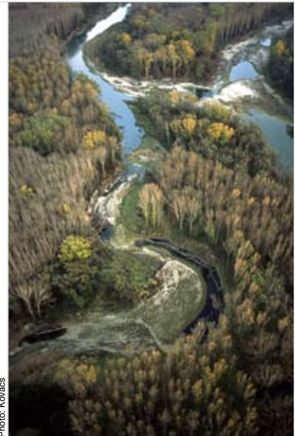
The impact of erosion after opening of the riverside branches (white area corresponds to new gravel areas)
